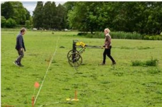
Running the Magnetometer
